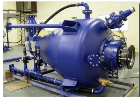
System 3 conveying vessel during assembly
