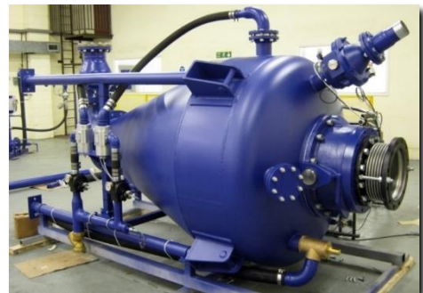
System 3 conveying vessel during assembly
